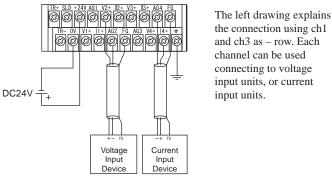
Ch 1 output voltage terminals V1+, AG1, FG Ch 1 output current terminals . .I1+, AG1, FG
